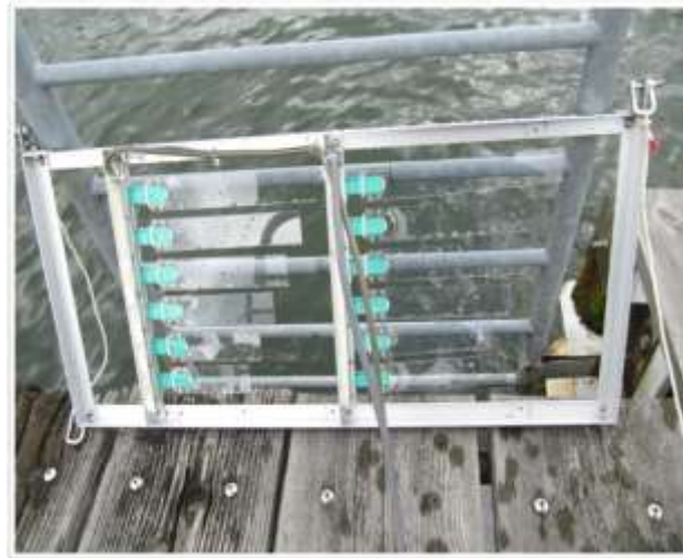
Fig.1 Small scale electric power system with piezoelectric elements (green boards) and flexible plates (transparent acrylic boards). Left side consists of six acrylic boards of 0.5 mm thickness and the right side has another six boards of 1.0 mm thickness. Six plates were spaced from top to bottom with lengths of 20 cm, 17.5 cm, 15.0 cm, 12.5 cm, 10.0 cm and 7.5 cm acrylic boards on both sides. The system was deployed into the water and each output was connected to an LED.
